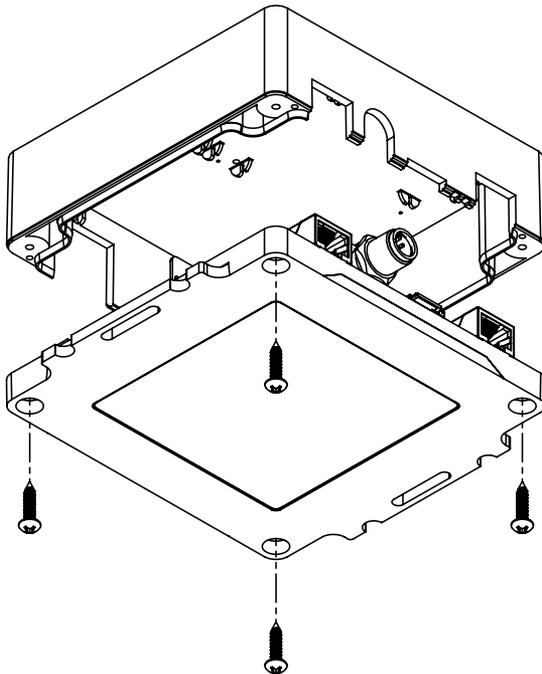
*Figure 5. LYNK II Case Construction*
