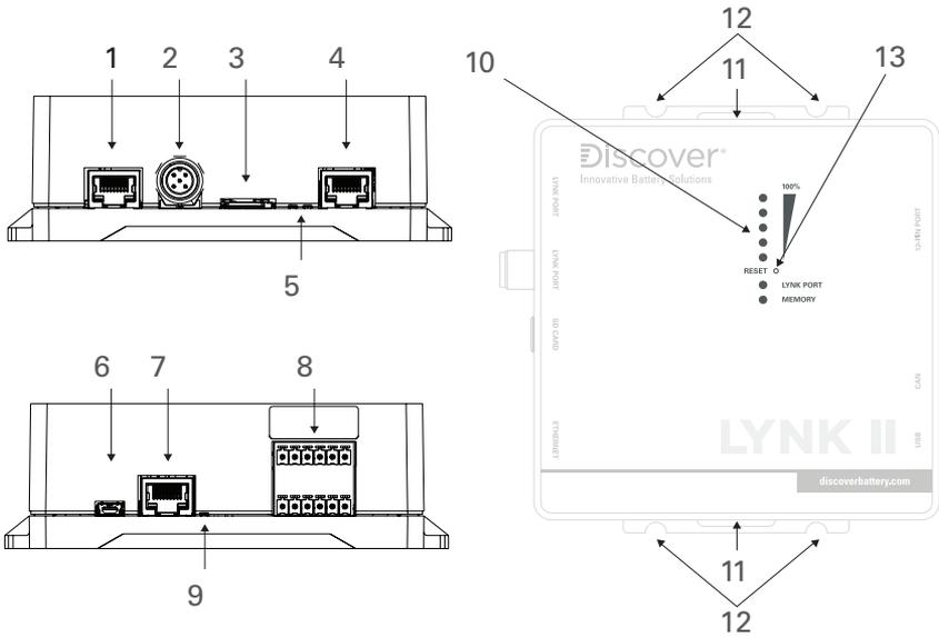
**Figure 1. Ports, Buttons, LEDs, and Mounting Hold Downs**
