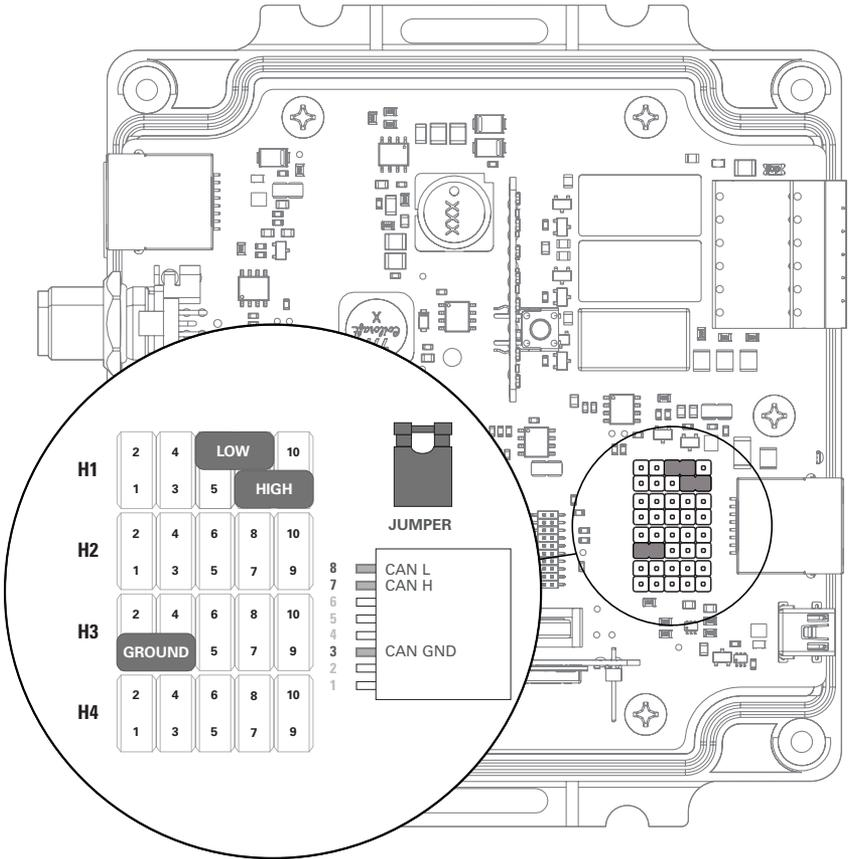
**Figure 8. Victron Energy and Studer Innotec PIN assignments**
