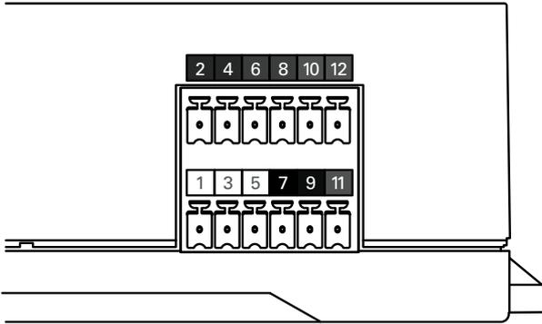
**Figure 4. PIN Assignments for Phoenix 12-PIN Connector**
