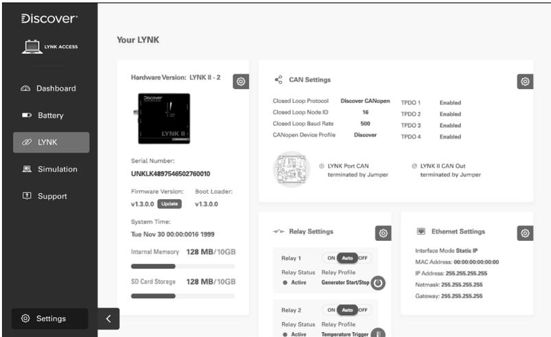
**Figure 18. LYNK II configuration and settings screen.**
