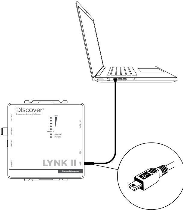
**Figure 17. LYNK II USB Type-B Mini connection.**
