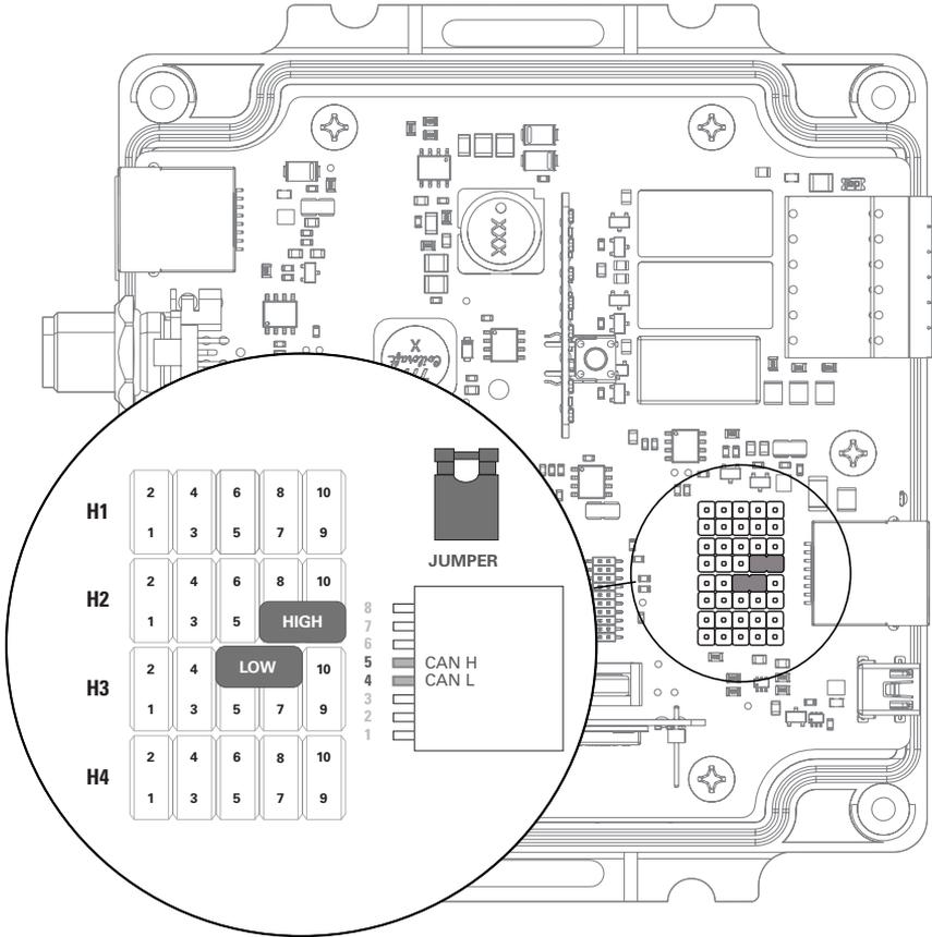
**Figure 9. Schneider Electric and Outback Power PIN assignments**
