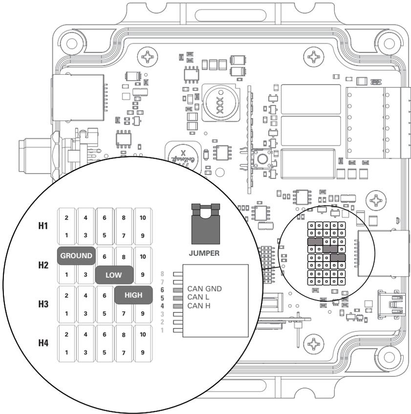
**Figure 11. Sol-Ark Outdoor CAN PIN assignments**
