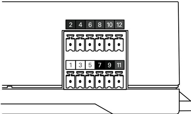
*Figure 16. PIN Assignments for Phoenix 12-PIN Connector*
