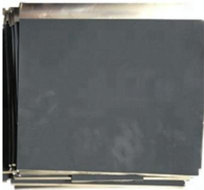
2. Generally, the negative electrode of conventional lithium cells is made from a carbon/graphite active material layer pasted onto a copper current collector negative(-) electrode (anode),
