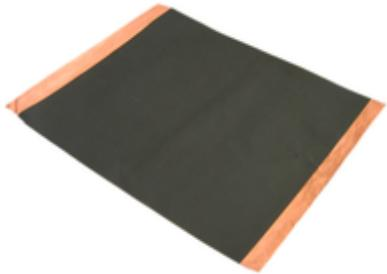
3. A separator that prevents the positive plate from coming in contact with the negative plate but porous enough to allow lithium ions to pass through as they migrate back and forth through the electrolyte solution during the charge and discharge process.
