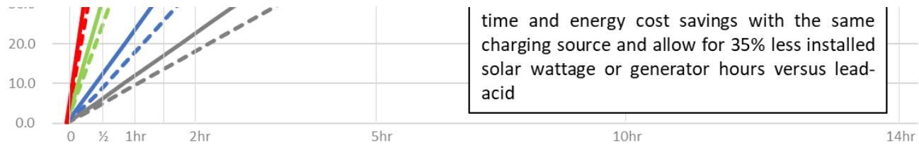
Lithium will charge to 98% SOC in the initial bulk charge stage and require short absorption time.
