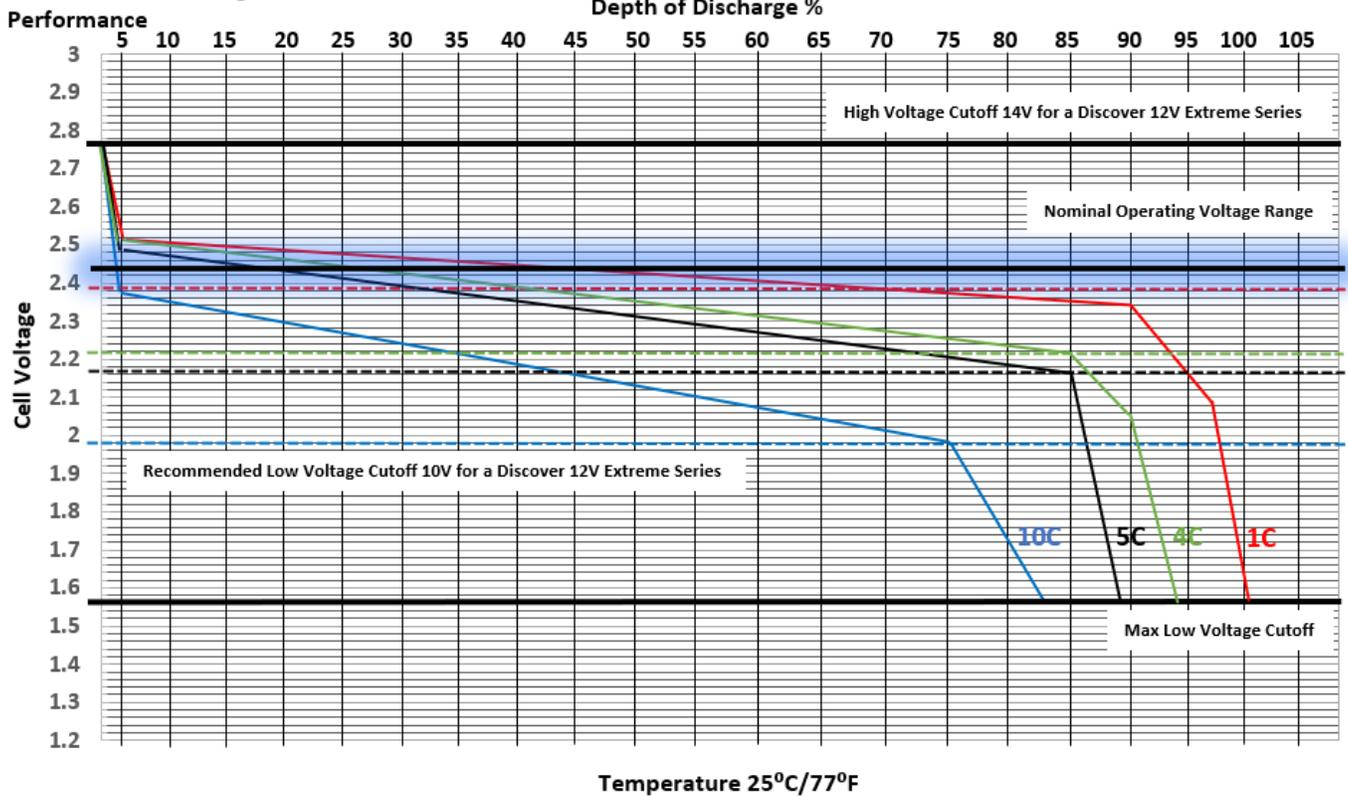
Discover's DLX lithium titanate batteries can be discharged at low temperatures
