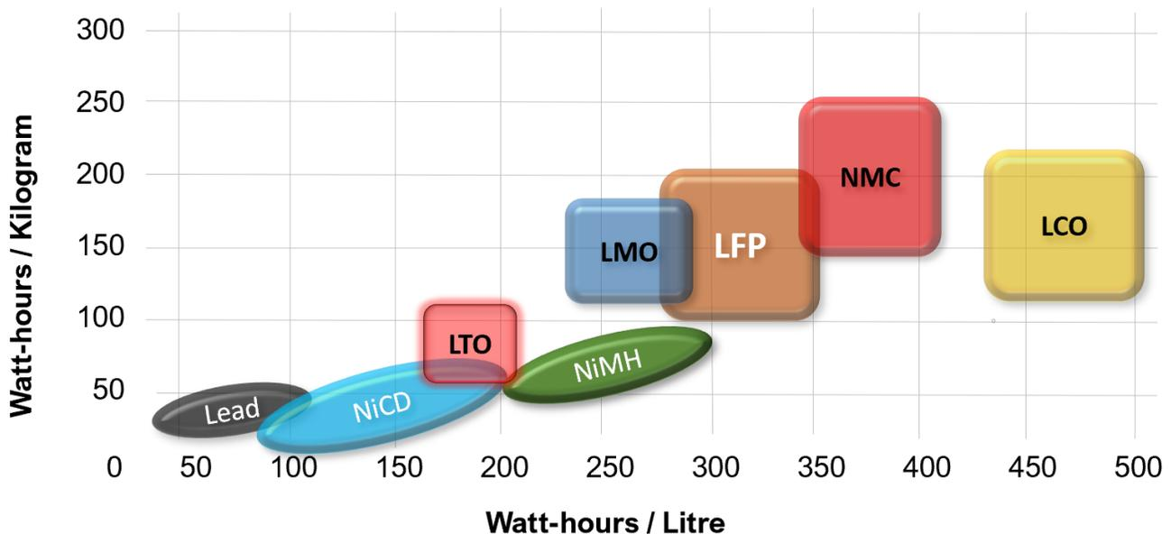
**High Energy Density means Higher Operating Voltage Means Higher Operating Pressure and Higher Operating pressure means Less Safety**
