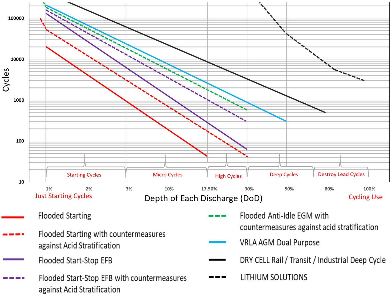
\*For various reasons high-energy lithium batteries are not generally suitable for starting use!
