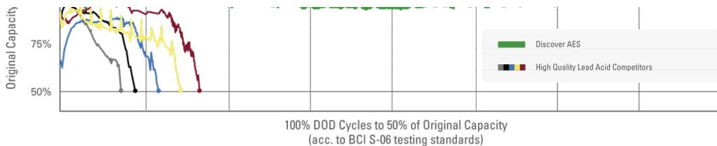
**DISCOVER LITHIUM SOLUTIONS to 100% DOD 1C x 1Hr rate discharges until the battery fails to deliver at least 60% of its original capacity above 2Vpc**
