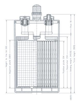
During assembling of OPzS blocks we need the bolted connection only between the end poles. All other poles of a block are also guided through the lid, providing sliding of the pole through the lid.
